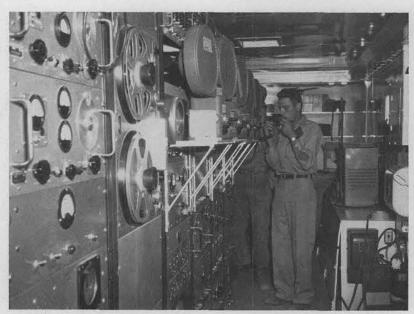
FINAL CHECK-OUT of telemetering equipment is made by Carroll B. McCampbell, 5222, as H-hour nears for a location field test.
